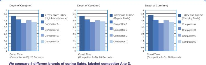
We compare 4 different brands of curing lights, labeled competitor A to D. In 20 seconds of curing time, their depth of cure is 4.6mm (Competitor A), 4.2mm (Competitor B), 4.5mm (Competitor C) and 4.3mm (Competitor D). The LITEX 696 TURBO cures a depth of over 5mm in 3 seconds (High Mode), 5 seconds (Ramping Mode) and 10 seconds (Regular Mode).
